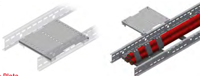
Smart Secure Plate Secure plates are highly recommended for fitting at the ends of trefoil cable runs. They provide additional support to reduce arching, deformation and stretch of the cables caused by short circuits.
