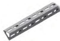
CH50-2T Triangle support channel Available in 1.5 and 2 mm material thickness. Option available with M10/M6 holes.
